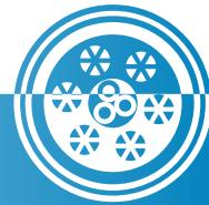
**Insulation Shield:** A semi-conducting thermosetting layer, applied in a triple extrusion process, plus a concentric serving of solid copper wires acting as both a drain wire shield and as a grounding (bonding) conductor—Black.
