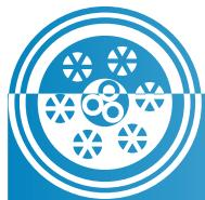
**Extruded Strand Shield (ESS):** Extruded thermoset semi-conducting stress-control layer over conductor.
